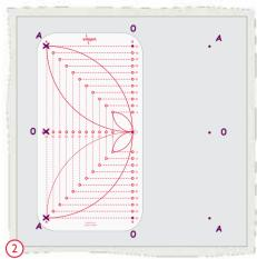
Flip the template horizontally. Make sure the vertical "0"- markings line up with the holes in the template. Put markings in the rest of the holes (marked 26), and do not forget to transfer the letters as well
