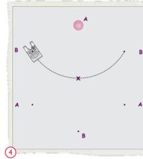
Set the Pivot Pin in one of the points marked "A". Sew from "B" through the center until you reach the next "B". Move the Pivot Pin to the next "A" point. Again sew from "B" through the center until you reach the next "B". Repeat for the last point marked "A".
