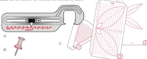
With the Circular Attachment, you can sew circles with a diameter measuring from 6 cm up to 26 cm (2<sup>1</sup>/<sub>2</sub> to 10<sup>1</sup>/<sub>4</sub>"). The diameters of the circles are printed in both centimeters and inches.
